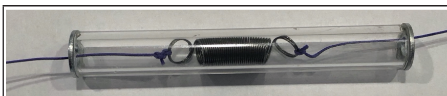
Figure 2. Spring device consisting of a thin spring inside a clear acrylic tube with washers on either end of the tube. The spring is tied to 0-vicryl suture on either end.
